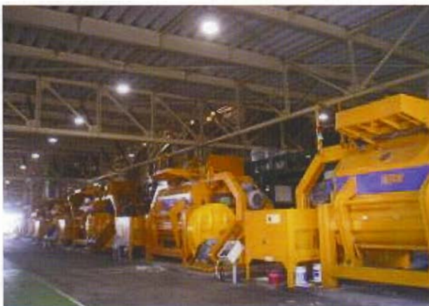
Preprocessing machines for crushing plastic waste into 30-mm-and-smaller fragments
