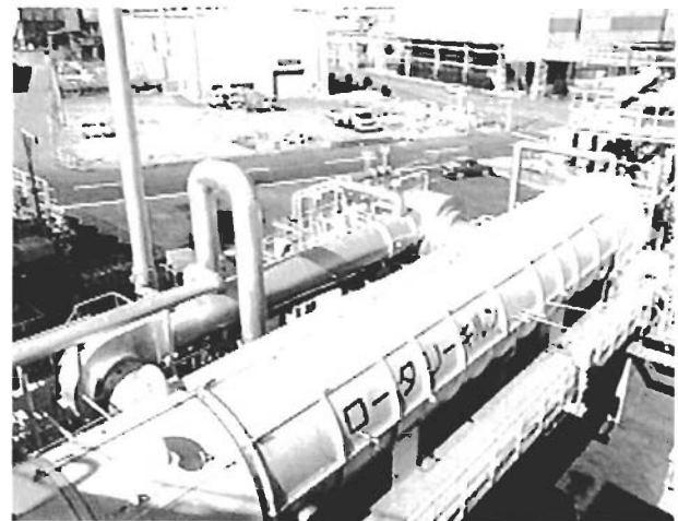
Rotary kiln for thermal breakdown of polyvinyl chloride into hydrocarbon and hydrogen chloride
