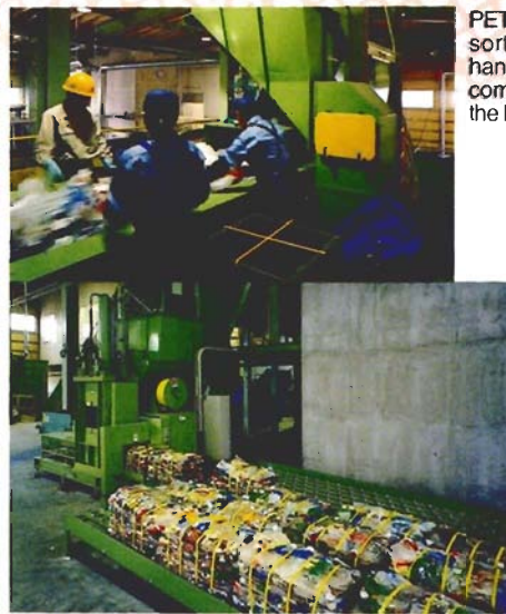
The compressed PET bottles are banded and sent to the recycling plant.
