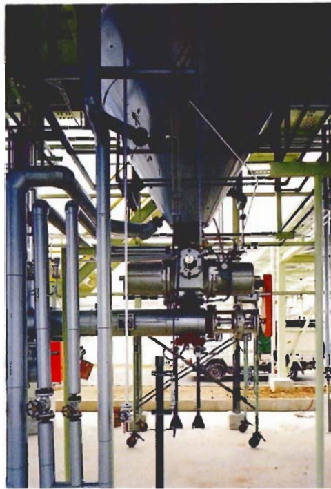
In this dehydrochlorinator, the polyvinyl-chloride resins in the plastic waste are heated and melted and the chlorine fraction is isolated in the form of hydrogen-chloride gas. The deaerator can be seen on the left.
