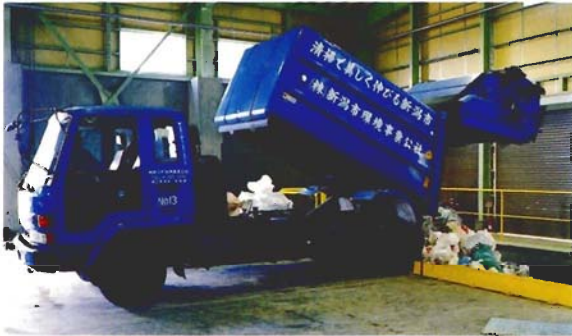
A sorted collection of plastic waste is dumped into the receiving hopper from a collection truck.
