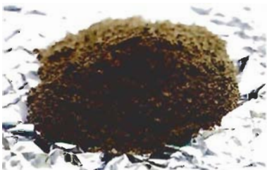
Ecocement is cement that is produced by the fly ash, sewage sludge, pastic waste, etc. Chlorine in Ecocement has the effect to shorten hardening time.
