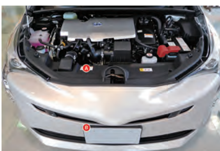
A Radiator support opening cover B Front bumper extension mounting Parts for automobile engine compartments Photo : ISONO Co., Ltd.
